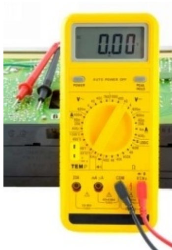
A typical DMM used for measuring current, voltage, resistance and many other electronic and electrical parameters
